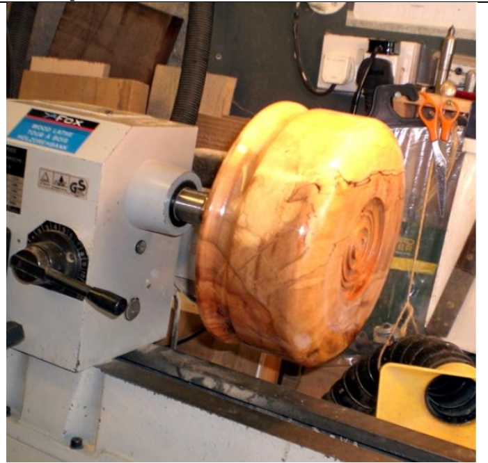
The outside has been sanded, sealed and a friction polish applied with a final coat of wax
