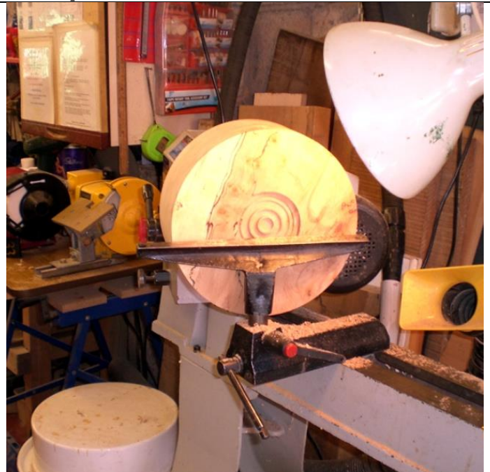
A recess is formed for a scroll chuck to be fitted
